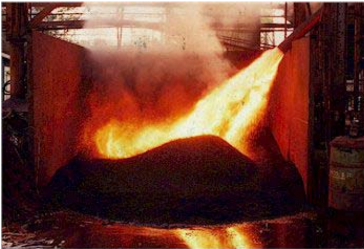
Figure 2: Hot sponge iron discharge into the open atmosphere. Fine product reacts with air and creates yellow flame.
