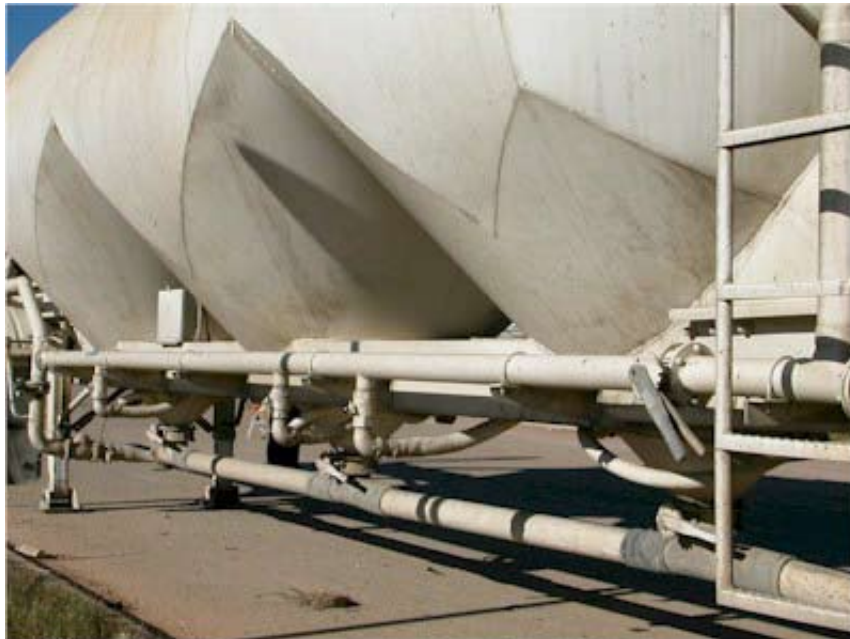
Figure 2: Pressurized Bulk Truck
